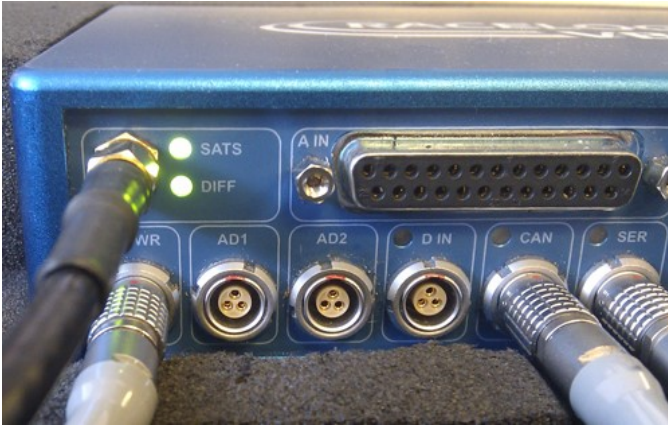
'DIFF' LED on the VBOX front panel is illuminated green.
