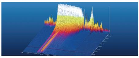
This figure shows an extract of High-Frequency-Impulse-Measurement (HFIM) signals of a cold forming process. During this process, steel sheets were formed to produce a vehicle body component. The HFIM-Piezo-Sensors were placed at the forming tool itself. The upper depiction shows a flawless forming process, the extract is limited to emissions which originated in friction between the steel sheet and the forming tool and plastic deformation.
